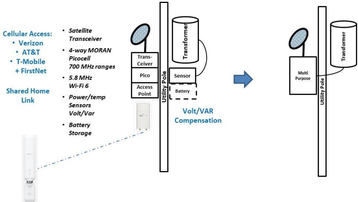
As the initial Direct Internet Access is being deployed, the back-office arrangements will be put into place to begin to use the neutral host multi-operator picocells for direct access expansions for the major carriers as well as local carriers as shown in the diagram below.
